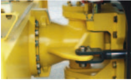
Maintenance-free, rugged, oscillating-articulation joint bolted on the outside of the front and rear frames
